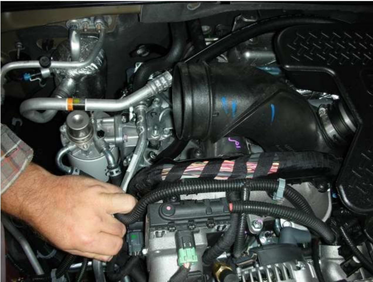
Here is the blue Finger Stick lead tapped into the harness ready for soldering. Use your wire stripper's 22 ga. Cutter to break the insulation and then just force the insulation away from the cut with your fingernails to open up enough room to tap into.
