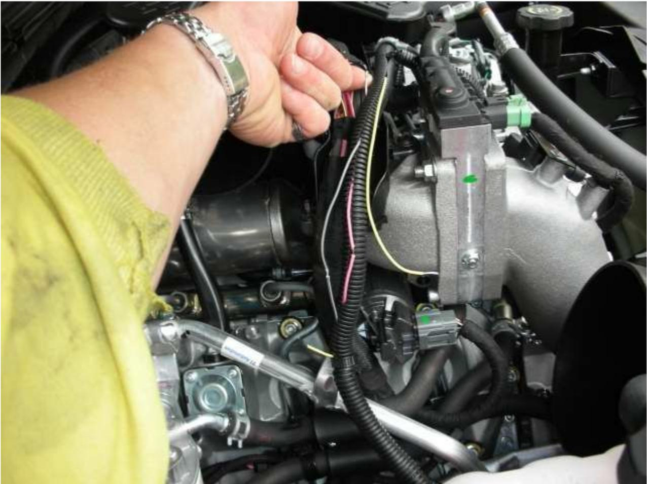
Notice that the joints on the Pink Gray and Yellow wires are staggered. This is so you don't end up with a giant bunch in your loom. (I hate bunches in my looms....)
